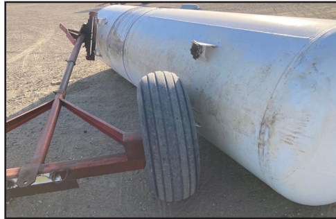
While moving this tank in a parking lot, a weld broke and the tank rolled off.
