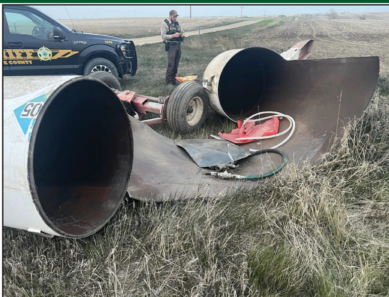
Had the anhydrous ammonia tank (above) been inspected per the Nurse Tank Inspection checklist (right) it might not have exploded, resulting in the death of a North Dakota farmer.
