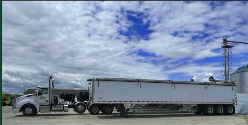
The dual-purpose, triple axle trailers kept fertilizer and grain moving this spring as needed. With application in full swing, they were equipped with unloading augers as fertilizer tenders. When the weather broke, augers were removed for grain transport.
